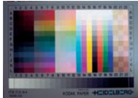
Kodak IT8 Test Target on color photographic paper. This is designed to profile how scanners render color.
