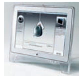
far left: X-Rite's Monaco OPTIX XR display calibrator. above: GretagMacbeth's Eye-One Display calibrator on an Apple LCD display.
